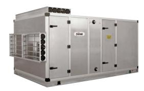
The panels are fixed to the frame with galvanised steel or stainless steel screws and are equipped with self-adhesive type seals. The inspection panels are fitted on hinges and provided with double closing handles (internal and external).
